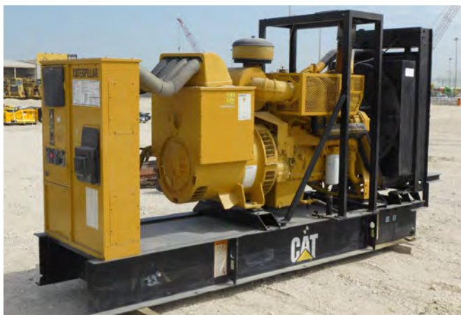
CAT LC6 365 KVA SKID MOUNTED
