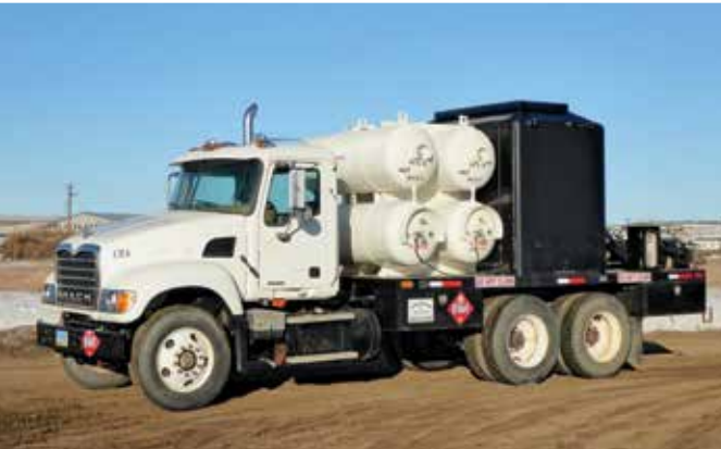
Mack CV713 Granite Heater
