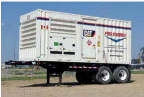
1 of 3 – Caterpillar XQ500 500 KW
