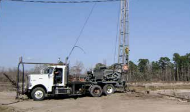
Freightliner Workover Rig
