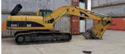
Caterpillar 322CL w/Labounty Shear
