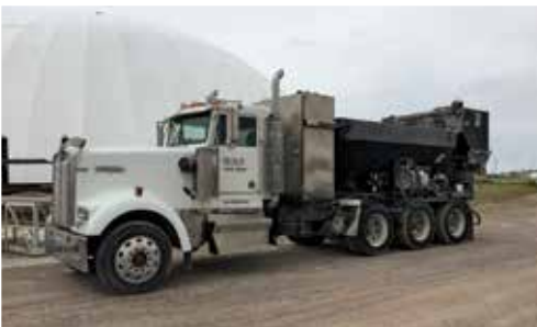
Kenworth W900 w/Mobile Mixer 710 Cu Yd Batcher
