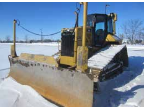
2012 Caterpillar D6N LGP w/Trimble GCS900 Minneapolis, MN
