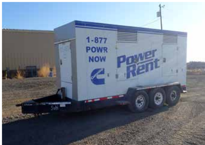
Cummins 350DQBB-360 350 Kw
